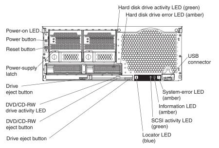
**Power-on LED:** This green LED turns on and stays on when you turn on your server, and it flashes when the server is in Standby mode.
